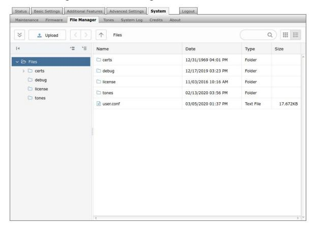
Files must be uploaded on to the designated folder, unless the 8190S will not recognize the file. For TLS provisioning and SIP signaling, a certificate file must be uploaded on to the 'certs' folder. Where as Informacast license has to be uploaded on to the 'license' folder. The 'tones' folder will be pre-loaded with audio files, more audio files maybe uploaded.
