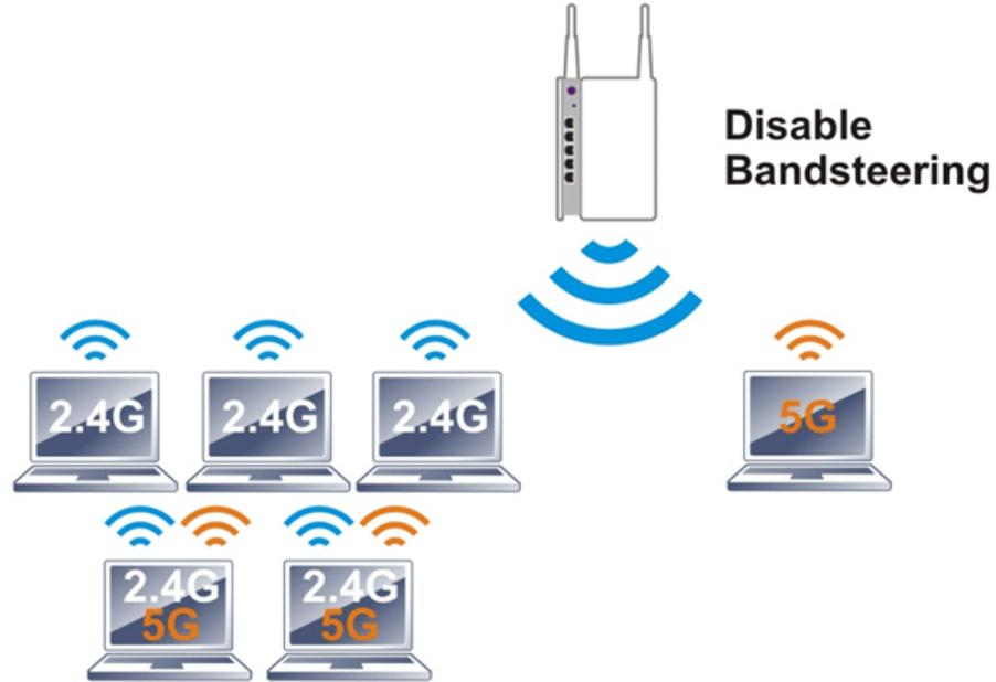
If dual-band is detected, the AP will let the wireless client connect to less congested wireless LAN, such as 5GHz to prevent from network congestion.
